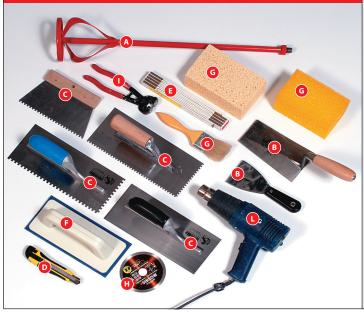
**EQUIPMENT** (A) Helicoidal whisk to mix binder and sealer (B) Stainless steel squeegees and trowels (C) Smoothe squeegee, stainless steel square tooth mm 3 and mm 5 (D) Cutter (E) Measuring set (metre, pencils, ruler) (F) Rubber plasterer's trowel to flatten and plaster sheets (G) Cellulose sponges set fit for cleaning epoxy materials (H) Continuous gear diamond lapping wheel placed on angular sanding machine (I) Pincer for manual cutting fit for glass (L) Fan for adhesive film removal.
