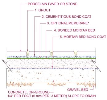
\* USE OF A MEMBRANE IS OPTIONAL. SEE TCNA MEMBRANE OPTIONS. SCALE: N.T.S.
