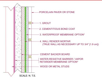
\*USE OF A MEMBRANE IS REQUIRED (WATERPROOF, WATER-RESISTIVE BARRIER OR VAPOR RETARDER) SEE MEMBRANE OPTIONS IN CURRENT TONA HANDBOOK
