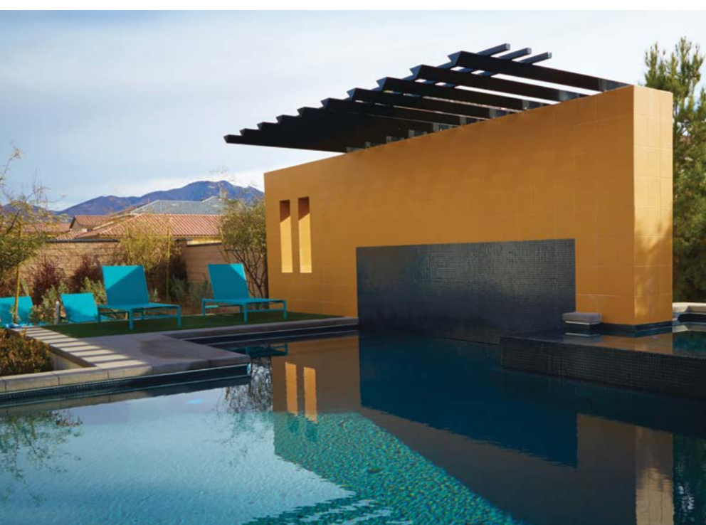
Per the TCNA Handbook, any submerged glass mosaics must be face-mounted.
